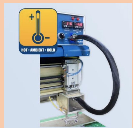
Thermal test w/Exatron. Wide Range Thermal Head -55°C to +155°C
