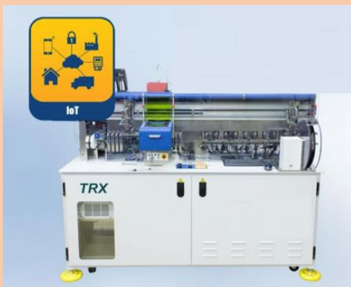
IoT device programming, serialization and laser mark - up to 2400 units per hour
