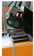
vision inspection module includes a Keyence vision sensor that can manage OCR/OCV for readability of text, numbers, logos verification, bar code verification (1D, 2D like QR magnetic code), stripe detection, chip detection, etc.
