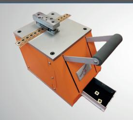
The **Spu 20** manual punching system allows getting a chip, a contact plate or a fingerprint sensor out of a 35 mm reel, one by one.
